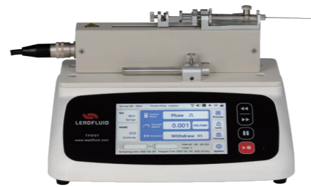
TFD01-01 SYRINGE PUMP Syringe: 5µL~1mL Flow Range: 0.058nL/min(5µL)~1.587mL/min(1mL)
